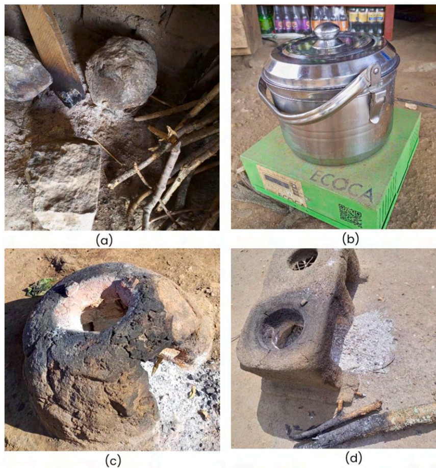
Fig. 11. Cook stoves used: (a) 3-Stone stove; (b) Solar electric cooker; (c) Single spot lorena stove; (d) 2 Spot lorena stove.
